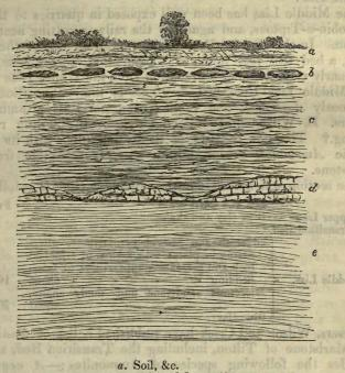
a. Soil, &c. Upper Lias b. Fish and Insect limestones. c. Clays. Middle Lias d. Marlstone Rock-bed. e. Clays, &c.
