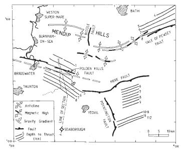
*Figure 4.* Map of postulated thrusts south of the Polden Hills and the Mere Fault in relation to the Poyntington Fault. (From Donato, 1988).
