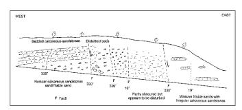
*Figure 2.* Sketch section showing dislocated Bridport Sands in Gore Lane, Nether Compton, Dorset.
